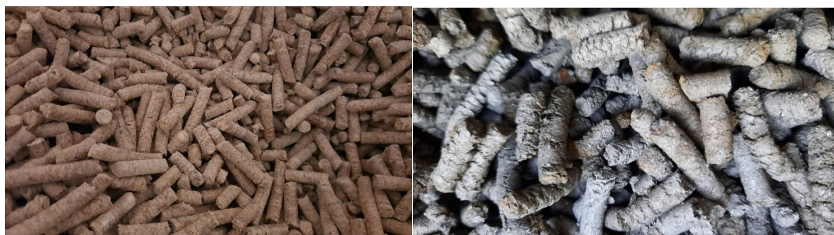
Fig. 1. Left: pelletized dried food waste as feedstock before TP, right: biochar after TP.
